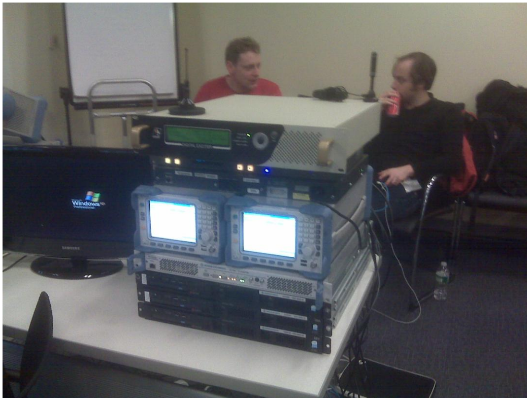
The Linear AT7001 M/H ATSC A/153 Digital Exciter interfaced with the Rohde & Schwarz AEM100 Multiplexer at PlugFest 2 confirming the S.5 Standard (proposed).
